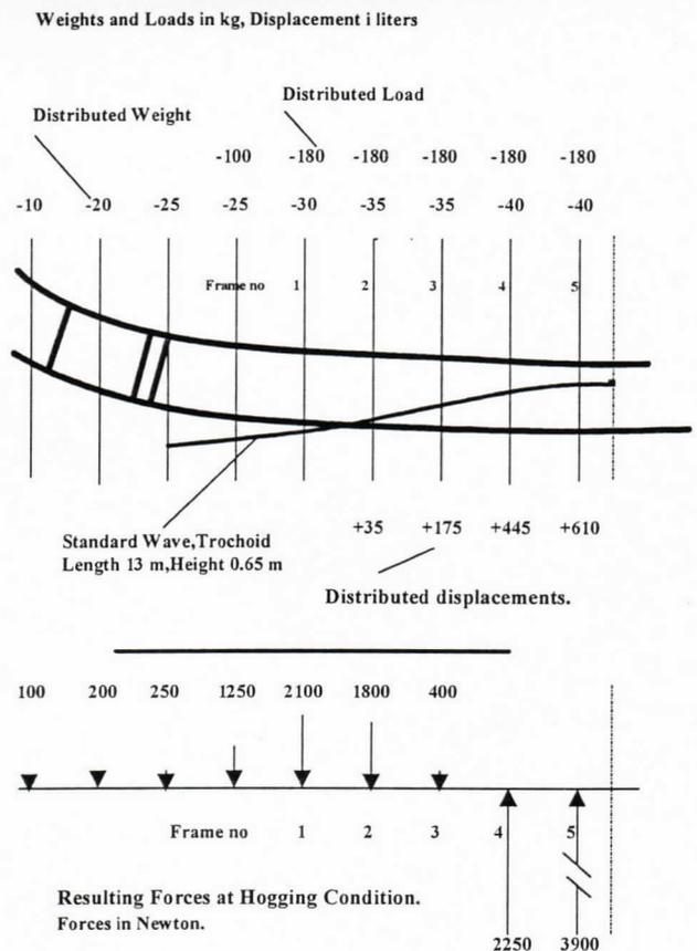
**Figure 14. External Forces at Boat Hull.**
