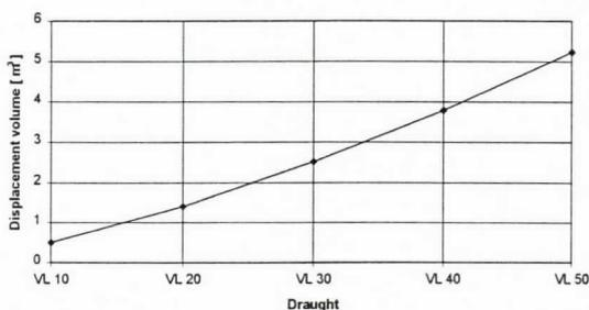
Figure 3. Displacements at Different Draughts.
