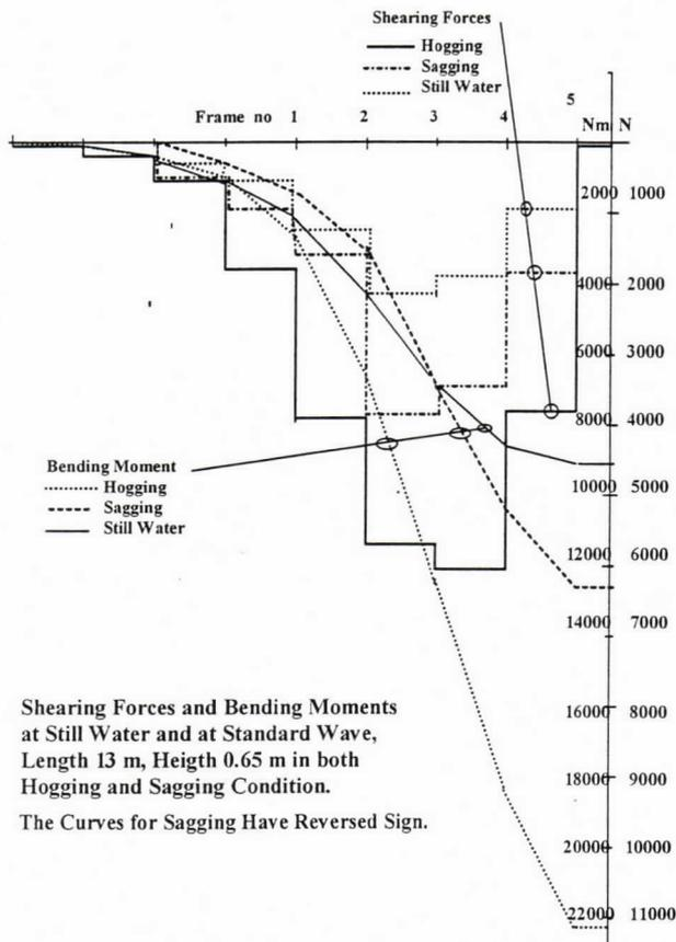
Figure 15. Internal Forces in Boat Hull.
