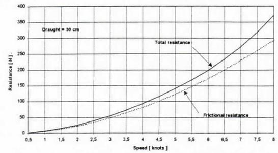
**Figure 8. Resistance of Propulsion**
