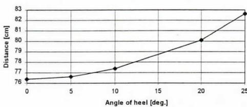
Figure 6. Positions of Metacentres above Bottom at Displacement 2.5 m<sup>3</sup>.
