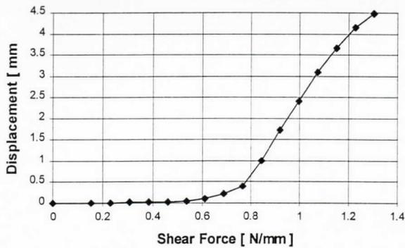
**Figure 13. Displacement vs. Shear Force of a Seam.**
