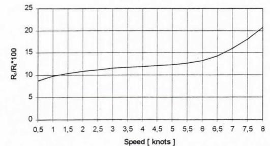
**Figure 9. Residual Resistance i % of Total Resistan**
