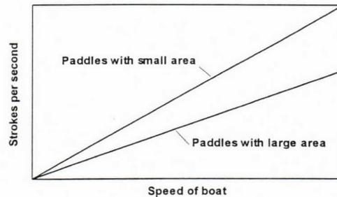
Figure 12. Paddling frequency vs. Boat speed
