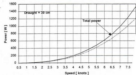
**Figure 10. Effective Power of Propulsion (at ment 2.5 m<sup>3</sup>)**
